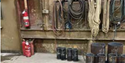
Welder qualification sample pieces waiting to be x-rayed
